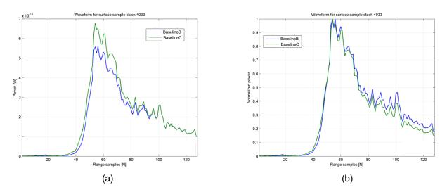
**Fig.16** Comparison of 20Hz level1b waveforms for BaselineB and BaselineC using the two different approaches for coarse slant range correction.
