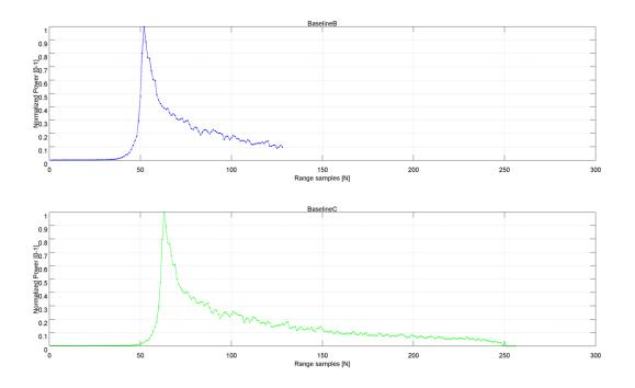
Fig.6 Examples of BaselineB SAR 20Hz waveform (128 samples) and doubled length of BaselineC SAR 20Hz waveform (256 samples).
