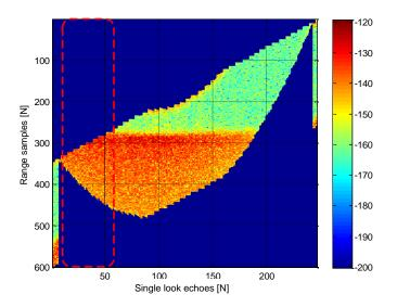
Fig.14 Surface Sample Stack with missed leading edge in some single look echoes.
