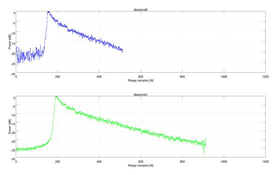
Fig.8 BaselineB and BaselineC SARin 20Hz waveforms in dB.
