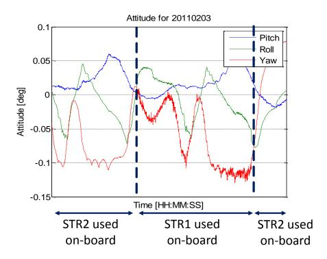
Fig.4 Example of attitude information produced by Star Tracker Processor.
