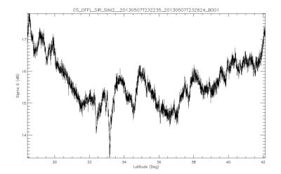
Fig.21 Sigma0 in dB obtained from SARin BaselineB product.
