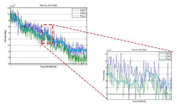
Fig.5 Example of mispointing angle in correspondence of a Star Tracker switch.
