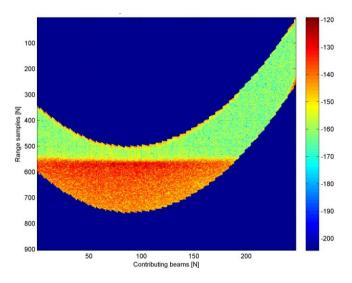
Fig.15 Surface Sample Stack with leading edge in all the single look echoes.
