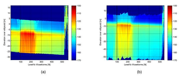
Fig.25 Close-up view on sample SAR product: z-scope for BaselineB (a) and BaselineC (b), colorscale in dB.
