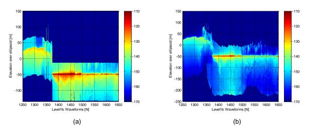
Fig.32 Close-up view on sample SARin product: z-scope for Level1b power for BaselineB (a) and BaselineC (b), colorscale in dB.
