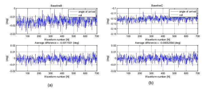
Fig.39 Comparison of roll angle and angle of arrival derived from the phase difference: BaselineB (a) and BaselineC (b).
