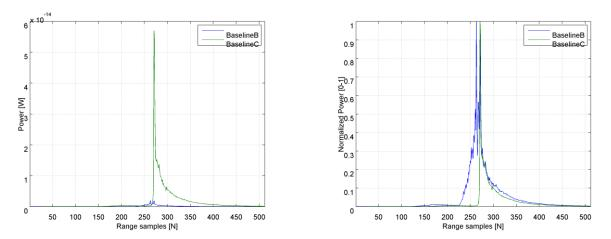
Fig.2 Comparison of BaselineB and BaselineC SARin 1Hz waveforms over ocean: Power (a) and Normalized Power (b).
