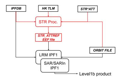
Fig.3 Block scheme of the Star Tracker Processor.
