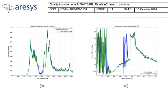
**Fig.13** SARin waveform by filtering out the ambiguity in case of complex return from the ground. In Fig.13(a), the dotted red line indicates the boundary of the applied rectangular weighting window.
