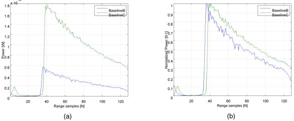
Fig.1 Comparison of BaselineB and BaselineC SAR 1Hz waveforms over ocean: Power (a) and Normalized Power (b).
