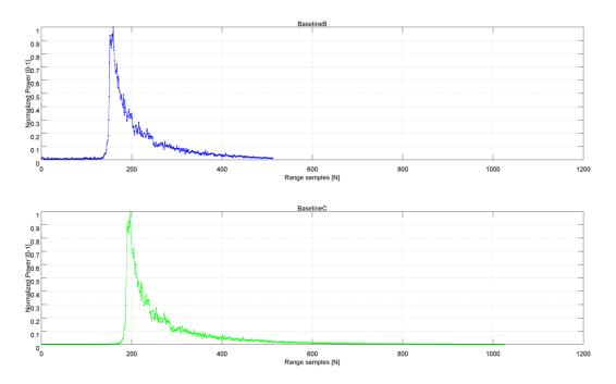
**Fig.7** Examples of BaselineB SARin 20Hz waveform (512 samples) and doubled length of BaselineC SARin 20Hz waveform (1024 samples).
