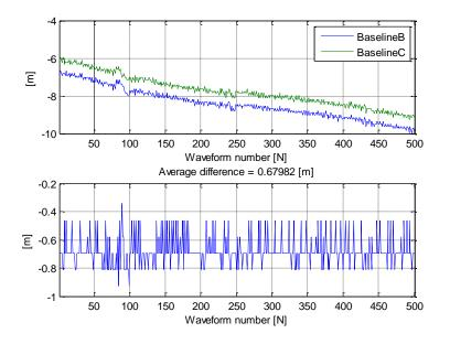
Fig.27 Retracking point for sample SAR product: close up view when sea is overflown.
