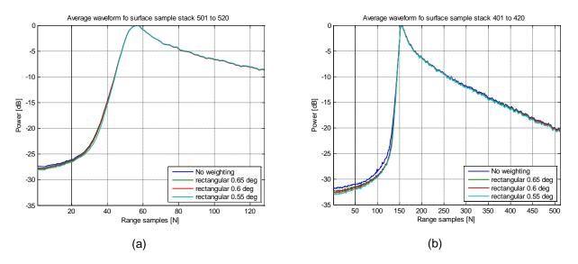
Fig.11 Averaged 20Hz Level1b waveforms for different values of  $D_w$ : SAR (a) and SARin (b).
