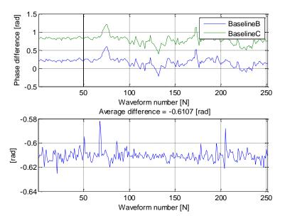
Fig.35 Phase difference at retracking point for sample SARin product: close up view when sea is overflown.
