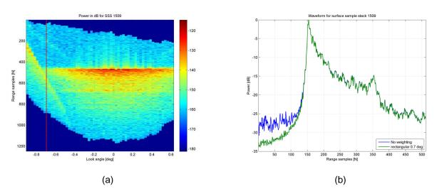
Fig.12 SCNR improvement on SARin waveform by filtering out the ambiguity. In Fig.12(a) the dotted red line indicates the boundary of the applied rectangular weighting window.
